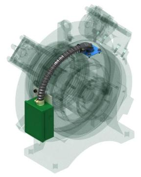
Figure 24: Factory Side Mount Electrical Box Relocation Example. Field Kit Available
